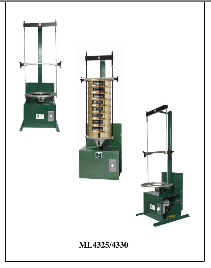
Thank you for purchasing the ML-4325 sieve shaker. You and your company will have many years of use from this quality testing system. This sieve shaker has the ability to accommodate a variety of sieves from 3 inch up to 8 inch diameter or metric equivalent.
